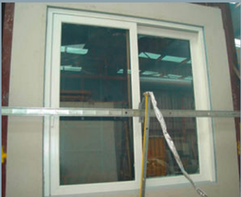
Unexposed (Inner) face of a Kömmerling PremiDoor after a BAL 40 AS 1530.8.1 Bushfire Resistance Test
