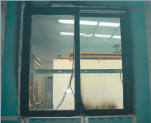
Exposed (Outer) face of a Kömmerling PremiDoor after a BAL 40 AS 1530.8.1 Bushfire Resistance Test
