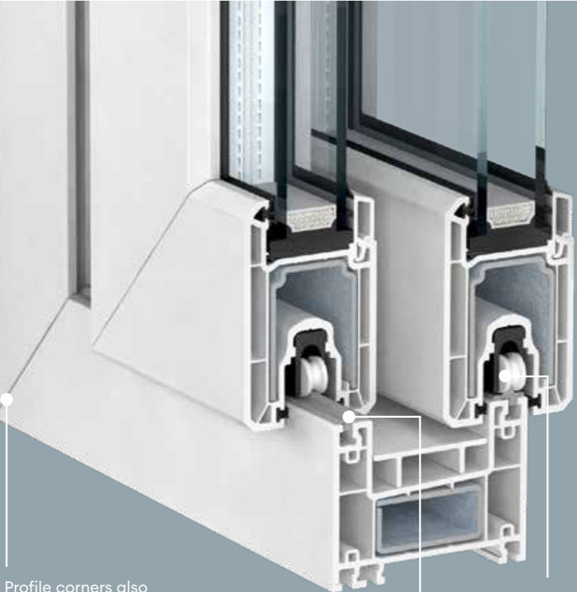
Thanks to rollers of special rigid PVC, the system promises exceptional quiet running and ease of operation
